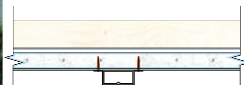
4. Gutter Fixing - Page 47
