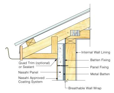
DETAIL 4.3 - Eave Detail (Panel Flush With Lining)
