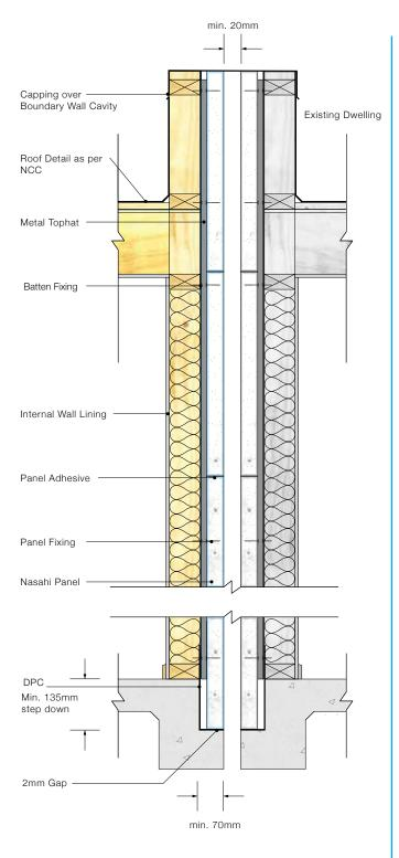
DETAIL 13.1 - Boundary Wall Detail (Even Slab)
