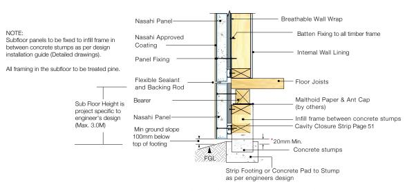
DETAIL 1.3A Sub-floor Infill Between Stumps (Also for sliding door sill)
