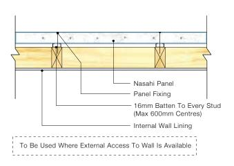
DETAIL 12.1 - Standard External Wall Detail
