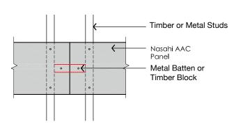
DETAIL 11.2 - Back Blocking for Missaligned Panel
