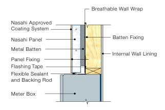
DETAIL 7.1 - Meter Box Installation
