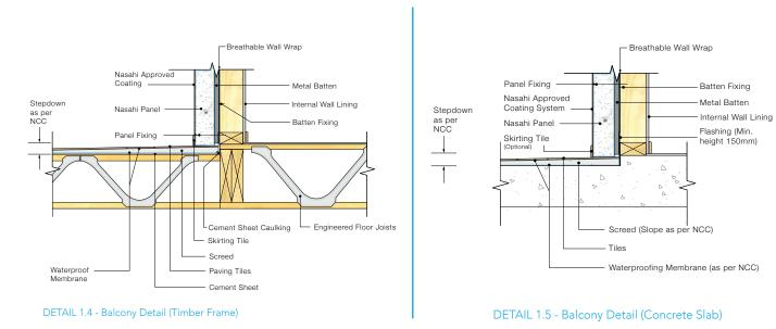
Note: On balconies if a 2mm cannot be provided between the bottom of panel and top of tile then weep holes at 1200 centres must be installed.
