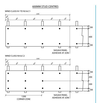
Note: Increase the number of fixing by 1 per batten in suspended applications.
