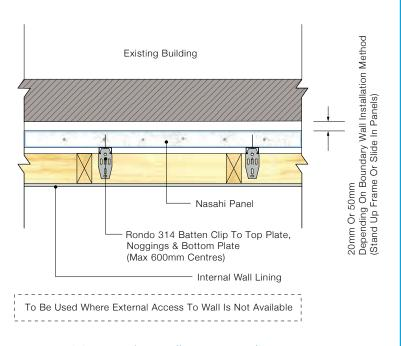
DETAIL 12.2 - Boundary Wall Fixing Detail B
