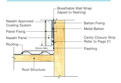
DETAIL 5.3 - Panel to Flat Roof Detail
