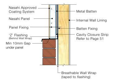
DETAIL 5.1 - Cladding to Brick Detail
