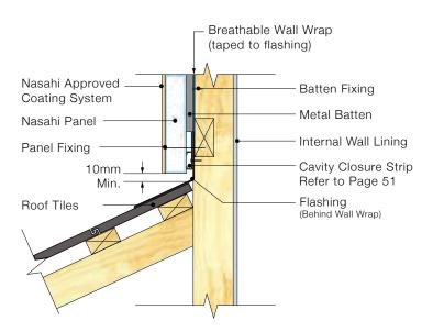
DETAIL 5.2 - Panel to Angle Roof Detail (up to 25°)
