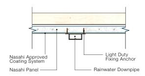
DETAIL 11.1 - External Fixings to Wall
