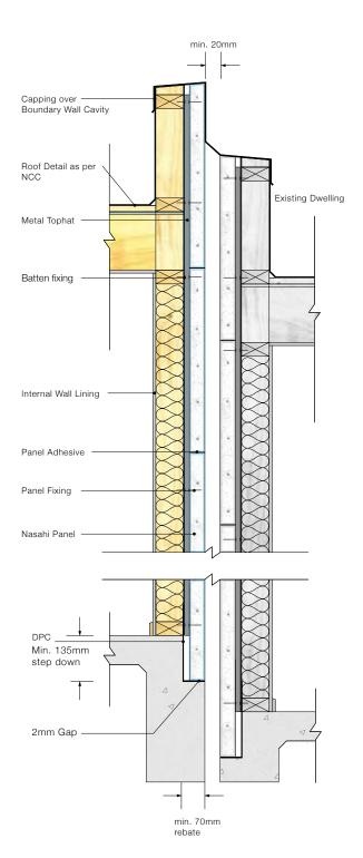
DETAIL 13.2 - Boundary Wall Detail (Uneven Slab)
