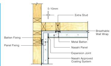
DETAIL 2.2 - Internal Corner Detail
