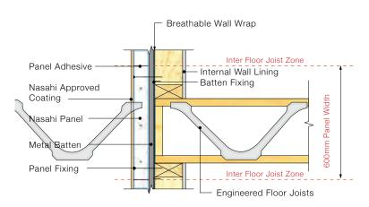
Note: To avoid control joint the joist must close within 600mm panel with Inter Floor Joist Zone
