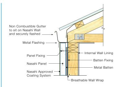
Detail 4.1A - Gutter on Boundary Wall
