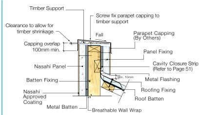
DETAIL 9.1 - Parapet Detail
