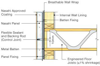
Note: For engineered floor joists, shrinkage ≤1% over depth of joist panel gap 5-10mm is acceptable. For non-engineered floor joists, panel gap of 20mm is required.
